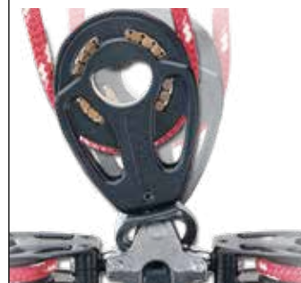
Control blocks attach to ears to reduce load on car.
