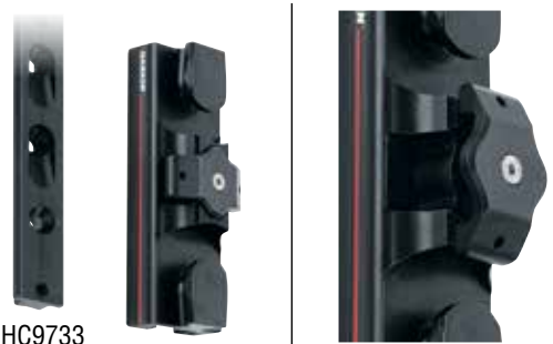
To lock pin in up position, pull the handle up with a lanyard or by hand and twist 90 degrees.
