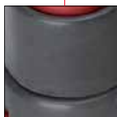
6061-T6 aluminum: Hard Lube-anodized
