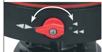
A simple flip of the red knob on the winch base turns on the rewind feature.
